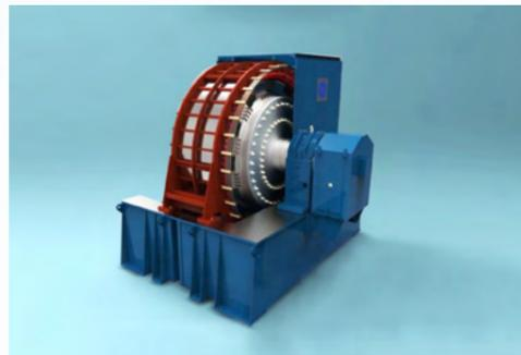
with a large mass to create as much inertia as possible. A rotating stabilizer can also generate and absorb reactive power and provide a large amount of short circuit current during transmission network faults, which helps with to stabilize the local voltage level during steady state and fault conditions. Statkraft is building two rotating stabilisers at Keith in Scotland, and this is scheduled for completion in the autumn of 2021.
